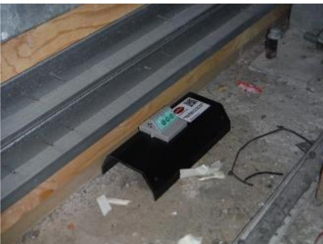
GT sensor mounted on upturned gutter
